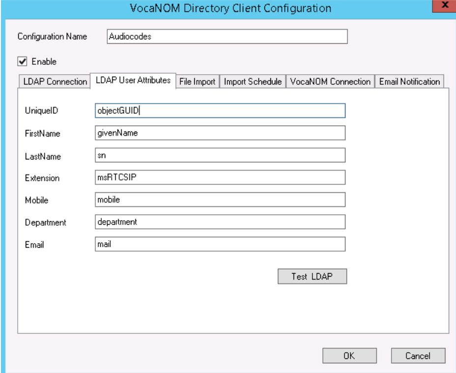
The screenshot shows the "VocaNOM Directory Client Configuration" dialog box. The "Configuration Name" field is set to "Audiocodes". The "Enable" checkbox is checked. The "LDAP User Attributes" tab is selected, showing the following fields:
